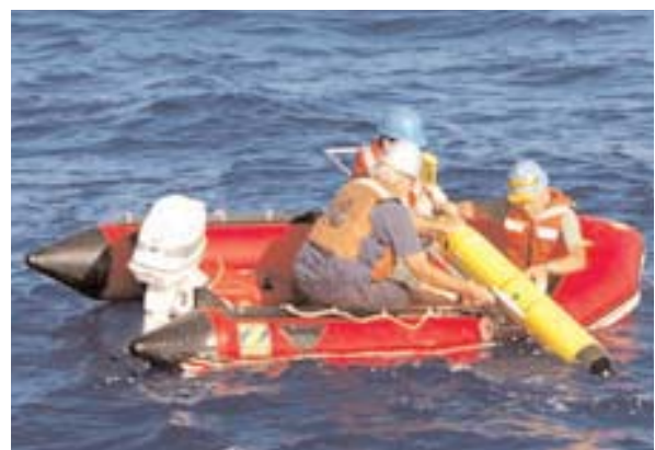
Ocean gliders are small, free-swimming vehicles that can steer to depths of up to 2000 meters.
